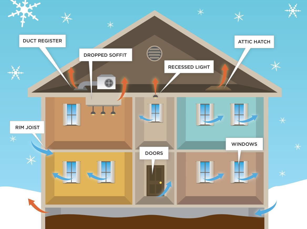
Properly air sealing your home, combined with upgrading your insulation will prevent the energy-sucking nature of the stack effect, and keep your home comfortable and energy efficient all year round.
